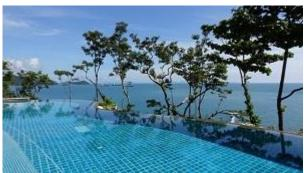
Typically found in luxurious resorts or hotel settings, an infinity pool features water flowing over one or more edge, giving the visual impression of merging with the ocean or sky. A 'weir' is constructed slightly below the pool level where the pool edge terminates. Below the weir, collects water spilling over the weir before being pumped back into the pool.
